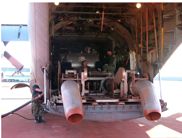
Plate 4 C-130 Hercules and MAFFS G-I showing lowered discharge chutes.
