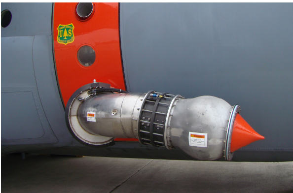
Plate 8 Shows the single dispensing chute and drop control valve.
