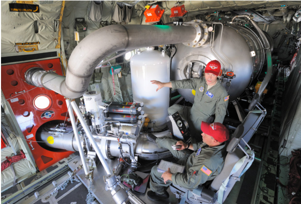
Plate 7 Internal fitment of MAFFS G-II inside C-130 Hercules, lower left of image shows dispensing manifold.
